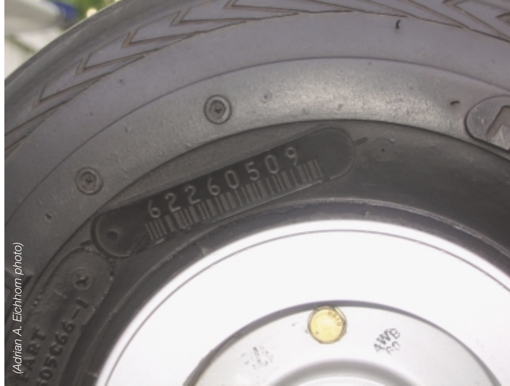
This barcode and number shows the date of manufacture for this particular tire. Different manufacturers use different coding to show when and where a tire was made. To avoid buying an "old," new tire, pilots should learn how to "read" tires.
